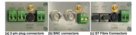
Fig 3. Power Input, Antenna Jack (SMA), Digital Outputs P3(A) & P2(B)
